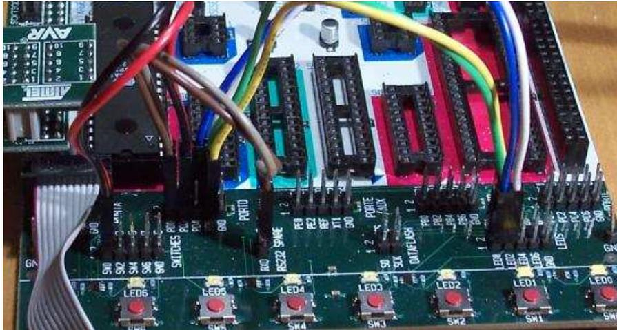
Figure 8: Wiring option #2 of the STK500
