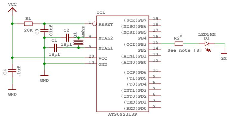
Figure 5: Schematic of circuit for demo project
