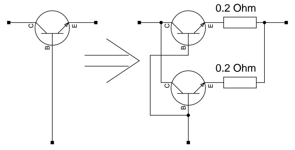
to use two power resistors instead of one you should add resistors in the emitter line to ensure even current distribution among the two resistors.
