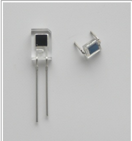
Photodiodes: left: Everlight PD638C, right: BPW34
